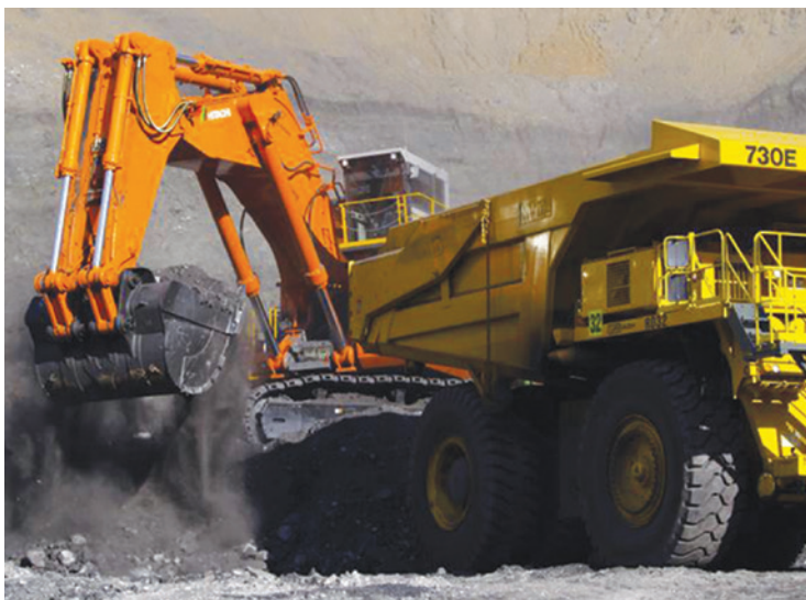
A Komatsu 730E truck is loaded by an excavator at the mine
